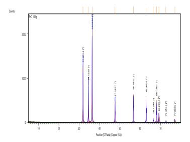
Figure 2. X-ray diffraction (XRD) pattern of ZnONPs as described in Mohamed et al. (2021).
